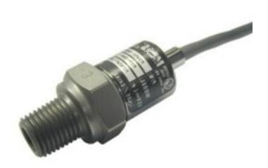
available. The Elite series single pressure transducers are available with standard pressure ranges of 0 to 500, 3000, or 5000psi. Additional pressure ranges are available upon request. Standard pipe threading is 1/4" NPT with alternative threading available upon request. The sensors have an accuracy of  $\pm 1\%$  full scale.
